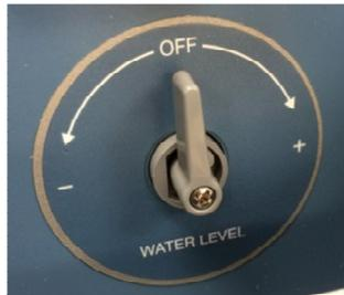
4. When processing actual samples – and the tube rack and samples are installed into the cup, the water level will require adjustment. See page 16.
