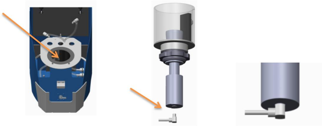
Note: the front area of the cup horn is clear. There is a horizontal line etched across the back side.
