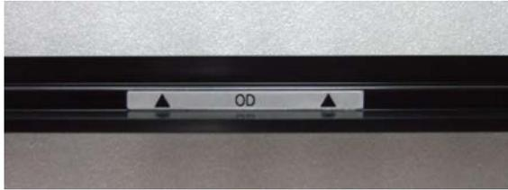
The spacers are placed by hooking them onto grooves on the floor stage. Refer to [Spacer positioning, on page 51](#) for more information about positioning the spacers.
