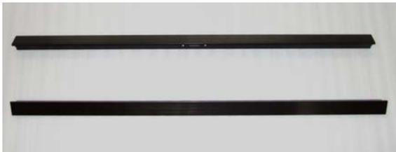
The digitization/OD spacers can be used both for digitization and for OD measurements, depending on the orientation and placement of the spacers. The illustration below shows the orientation in which the spacers are used for digitization.
